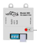
The LED blinks red when the module is broadcasting its WiFi network. Once connected to the home network the LED will be solid green.
