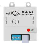
If the homeowner is ready to proceed with Wifi setup, push the WiFi switch on the iM3 WiFi module to broadcast the iM3 WiFi network. The module will broadcast its WiFi network for 30 minutes.
