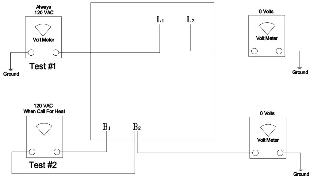
1. Using your meter, check voltage between L1 and ground. You should have 120 volts all the time. If you do not have 120 volts all the time, the wiring is wrong or your breaker is off.
