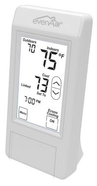
The EvenAir wireless, remote control thermostat controls whole house fan or economizer operation for free cooling. The TSRC can be wall mounted using the subbase supplied or on a table top using the table top adapter provided. The TSRC can turn Econo Cooling On or Off and set the temperature for cooling. The TSRC requires the ER1, Electronic Receiver Module, to be installed in the wiring hub.
