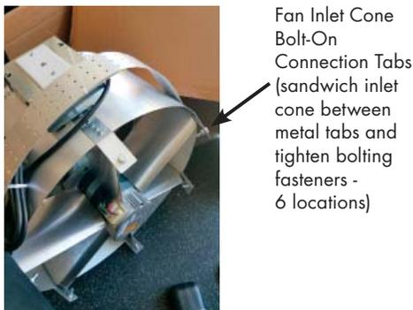
FIGURE 8 - Fan Assembly showing mounting tabs for Fan Inlet Cone
