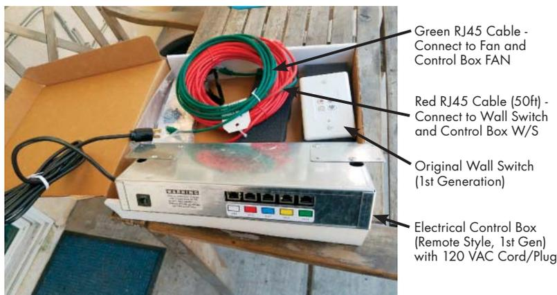
FIGURE 2 - Remote Mount Electrical Control Box
