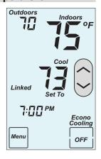
When the system is in Cool or ECool and the setpoint temperature is adjusted on the TSRC remote control, the new setpoint is automatically updated on the EvenAir thermostat. Similarly, when the setpoint temperature is adjusted on the EvenAir thermostat, the setpoint is automatically updated on the TSRC remote control.
