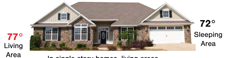
In single story homes, living areas with sun exposure feel too warm during the summer
