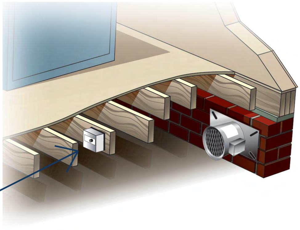
*Note: The de-humidistat is designed to be installed remotely, so it can be placed in the crawl space where moisture is most likely to accumulate.*
