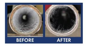
Calcium and magnesium particles tend to stick to each other and any surface they contact, forming layers of hard scale. This scale buildup damages water heater elements and restricts water flow. ClearWave reduces these particles. Once treated by the ClearWave Water Conditioner, calcium and magnesium particles remain in suspension, flowing freely through the system and down the drain.
